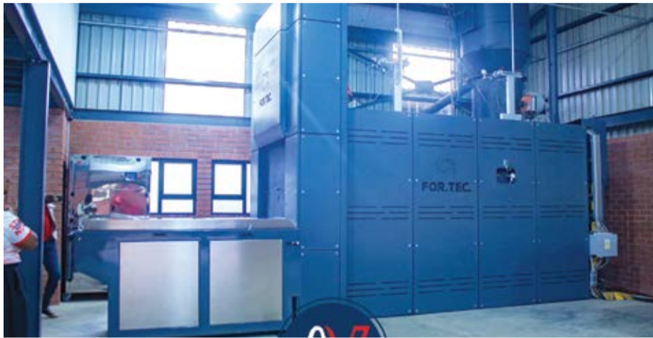
Inside New Dawn's crematorium, showing the high-temperature furnace used to cremate bodies.
